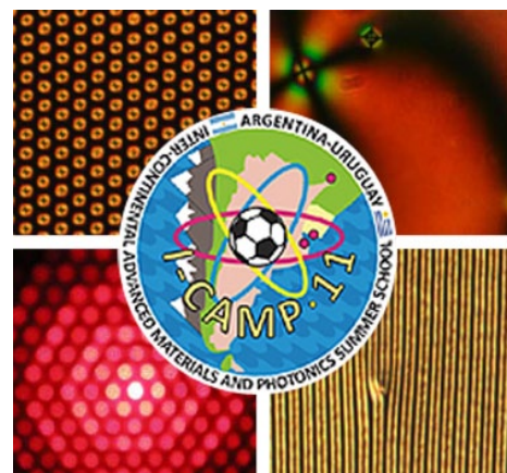
(top left and bottom right) Optically generated photonic structures in a cholesteric liquid crystal. (bottom left) A diffraction pattern obtained using a HeNe laser beam and a self-assembled periodic hexagonal structure. (top right) A nematic liquid crystal with topological defects and square-shaped colloidal inclusions.
